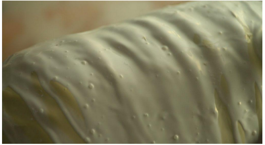
Bola, otherwise known as a Field Coagulated Latex Block- Latex coagulated naturally into basic forms of raw rubber.
