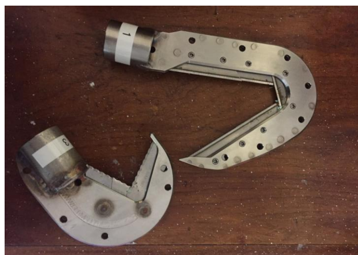
Image 14. Wayne Ledwell's disentanglement knives. The angles and gapes of these knives differ from the CCS ones. The serrated and smooth blades are interchangeable.
