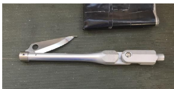
Image 12. This knife has been modified with an adjustable hinge, so that the knife can be angled when attached to a pole.
