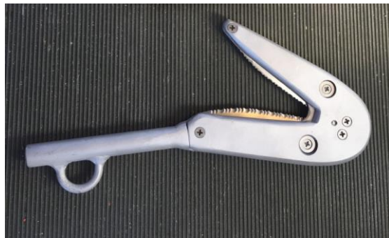
Image 10. an updated prototype ready for testing. This version has a wider gape for cutting thicker ropes, and replaceable blades which means only these need to be replaced when dulled, rather than the entire knife. The breaking strength of fishing ropes has doubled since the 1990s and therefore tougher knives are now essential to cut these.
