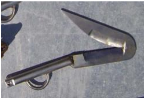
Image 9. An original welded one-piece flying knife that can be deployed using a pole and attached to lines on or trailing from a whale, to allow cutting to be done from a distance.
