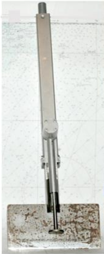
Image 15. A spring-loaded knife.
