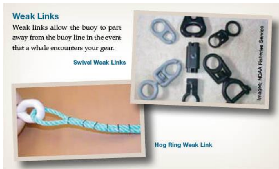
Image 22. Examples of weak link designs. Image credit: NOAA
