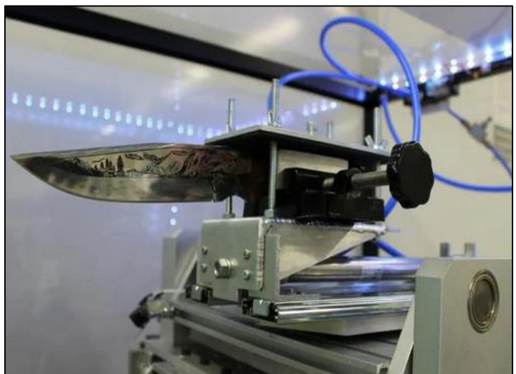
Image 42: The Conan stabbing machine developed between AFP, U of Canberra and UTS
